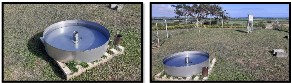
Figure 4.3: LEFT - evaporation tank and RIGHT - weather station at SRIF-Drasa.
