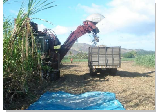
Figure 3. Track harvester in operation at Drasa Estate
