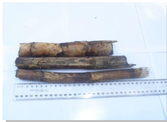
Figure 5. Irregular and damaged billets caused by poor harvester operations.
